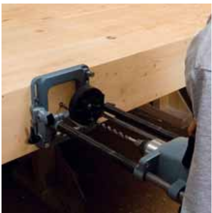
1. Pilot drilling with column type drill.
